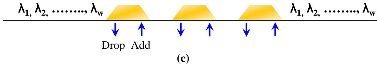
Serial, where wavelengths are dropped and added one at a time
