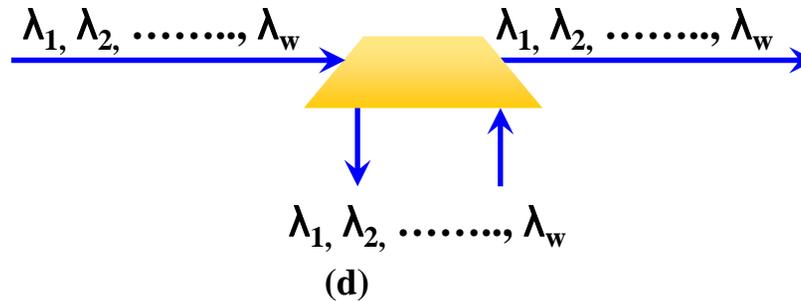
Band drop, where a band of wavelengths are dropped and added together.
