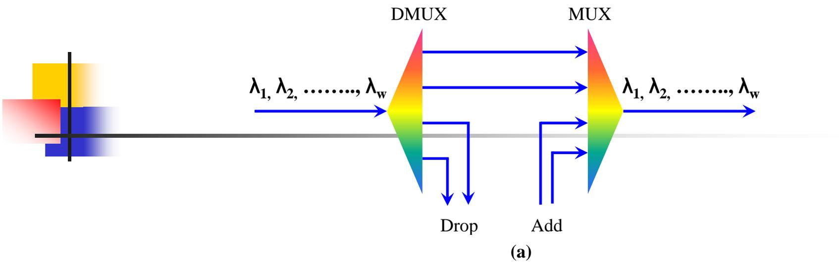
Parallel, where all the wavelengths are separated and multiplexed back
